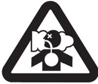
A generator's exhaust contains toxic carbon monoxide, which you cannot see or smell. Breathing carbon monoxide can **KILL YOU IN MINUTES**. To avoid carbon monoxide poisoning, follow these instructions when operating a generator:
